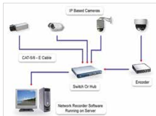
IP Based CCTV System with IP Camera, Video Management Software for on-line display of video images on monitor
